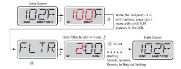
If Filter Cycle 2 is enabled, Filter 12 will appear in the LCD. If Filter is disabled, Filter 1 will appear.
