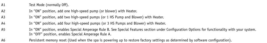
A2, A3, and A4 work in combination to determine the number of high-speed devices and blowers that can run before the heat is disabled. i.e. A2 and A3 in the ON position and A4 in the OFF position will allow the heater to operate with up to 3 high-speed pumps (or two HS Pumps and Blower) running at the same time. Heat is disabled when the fourth high-speed pump or blower is turned on.
