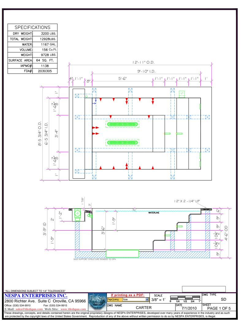
Voguebay MG02 Plain White Frosted 1"x1" - 180 sf #1 - FIELD TILE: Voguebay MG02 Plain white Frosted 2"x2" #2 - WATERLINE (optional): Voguebay MG02 Plain white Frosted 2"x2" - 26 sf #3 - TOP OF WEIR (6" waterline and top of weir) #4 - NO TILE ON LIP Date: #1 - GROUT: #2 - GROUT: #3 - GROUT:
