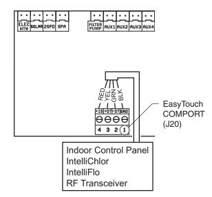
EasyTouch Control System Circuit Board
