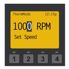
Setting the Thermal Mode Pump Speed
