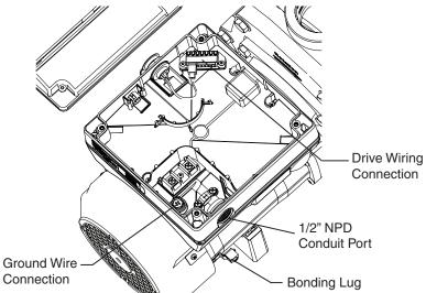
Field Wiring Compartment
