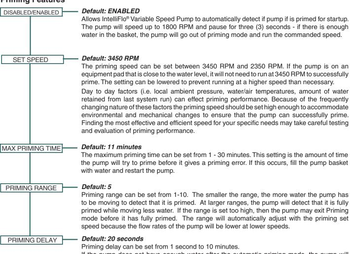
If the pump does not have enough water after the automatic priming mode, the pump will increase to the Maximum Speed (under "Pump Settings" on page 8) and run for 20 seconds (or for the time set).
