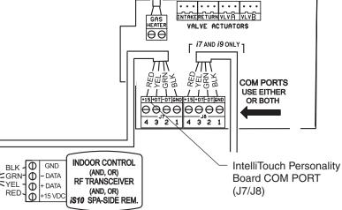
IntelliTouch Control System Circuit Board
