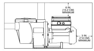
Figure 1: Pump Rear and Overhead Clearance
