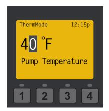
Setting the Thermal Mode Pump Temperature
