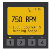
**Note:** The pump will not run the scheduled speeds until the **Start/Stop** button is pressed (LED on) to place the pump in Schedule mode.
