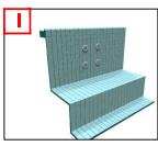
Water level line The highest recommended jet elevation is at least 3" below water level.
