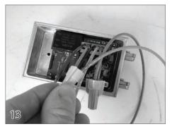
Continue connecting the power and directional wires to the pigtails on the controller using wire nuts.
