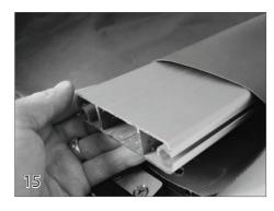
Insert the leading edge tube into the loop of the cover. Install the other side of the cover and slider.
