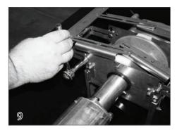
Raise the pulley brackets and the water side brackets level with the top of the encapsulation. Tighten the bolts for the brackets.
