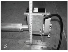
Attach the mechanism feet to the mechanism approximately 1 inch less than the distance from the bottom of the housing to the top of the track/encapsulation. Use a 7/16 inch ratchet to tighten bolts.
