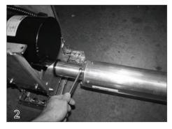
Attach the roll up tube to the motor end of the mechansim using the 3/8" x 1 1/4" bolts (36) and lock washers (37) provided.
