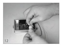
Connect the ground wires from the power supply, the motor and the ground wire from the touch pad together using a wire nut.
