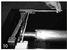
On the non-motor end, feed the rope around the pulley of the non-motor end pulley bracket. Pull the rope through to the motor
