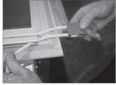
Wedge the rope into the back side of the track and pull through towards the housing. Insert the pulley end cap into the track. Repeat this on the other side of the cover.
