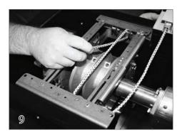
Pull the rope around the vertical pulley on the front wall of the housing.
