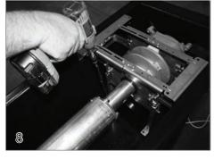
Attach the mechanism feet to the floor of the housing. Use the mounting hardware provided.
