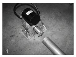
Assembling the mechanism. Turn the motor and non-motor end upside down. This is done to appropriately attach the roll up tube and the mechanism mounting feet.
