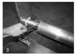
Attach the roll up tube to the non motor end of the mechansim using the 3/8" x 1 1/4" bolts (36) and lock washers (37) provided.
