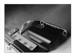
Install the black cap (10) over the top of the leading edge support bracket. Secure it in place by tightening the screws on the back side of the cap.
