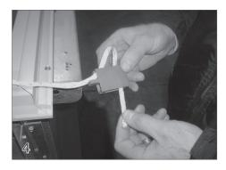
Feed the rope around the pulley end cap..
