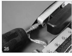
Attach the bonding wire to the leading edge bar using a self tapping screw (32).
