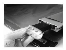
Insert the leading edge inserts into the leading edge tube.
