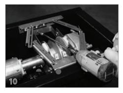
Attach the pulley brackets and water side brackets to the walls of the housing. Use the mounting hardware provided.
