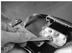
Attach the leading edge insert to the slider by inserting the a screw (41) from the bottom of the slider. The screw will go through a punched hole in the cover, then into the leading edge insert. Secure using a 10-32 Nylock Nut. (29)
