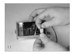
Connect the touch pad by wiring the neutral wire from the power supply, the white wire from the motor and the neutral wire that is connected to the touch pad using a wire nut.
