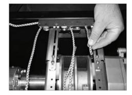
Feed the non-motor end rope behind the first and second and third horizontal pulleys.
