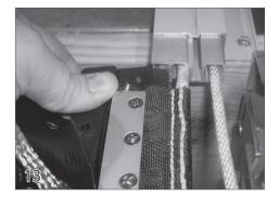
Feed one side of the cover and slider into the track.
