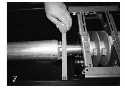
Center the tube in the housing. Tip: If the pool is not square, square up the mechanism with the track.
