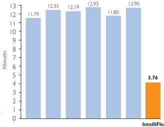
Data shows results of comparative energy use tests between IntelliFlo and six common pool pumps. IntelliFlo consumed between 68% to 71% less energy in every case. In actual use conditions, savings may be significantly larger:
