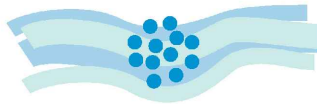
The Mod Media system strips away particles as small as 70 microns, (an average grain of beach sand is 100 to 2000 microns in diameter).
